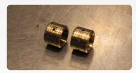
**Oil contamination:** The clearly visible grooves on the journal bearing surface arise from frictions and excessive material abrasion provoked by impurities in the oil. Despite the presence of oil, shaft of this turbo get seized.
