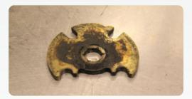
**Insufficient lubrication:** Oil coking on the thrust bearing – failure provoked by insufficient lubrication that caused overheating.
