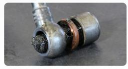
**Oil supply disturbance:** Severe oil contamination (sludge/carbonizing) caused oil feed line restrictions visible on banjo fitting.
