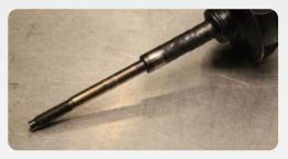
**Insufficient lubrication:** The surface of the turbo shaft is black and carbonized. Insufficient oil supply have caused overheating at first, thus making the steel color change. The blueish-to-yellowish color temperature is a heat tint caused by overheating of the shaft steel. Next, the remaining oil will start coking on the surface, making the black sinters.
