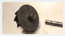
**Insufficient lubrication:** Broken shaft caused by lack of lubrication. The high rotation speed and frictions within the moving parts have caused the temperature to increase extremely, the shaft to warm up, and ultimately break by seizing.
